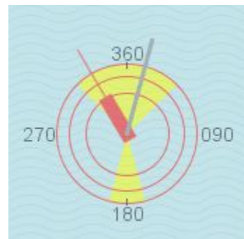
Bearing to mark: 360° Wind 10° (+10°) Lift up to 325° (+10°).
